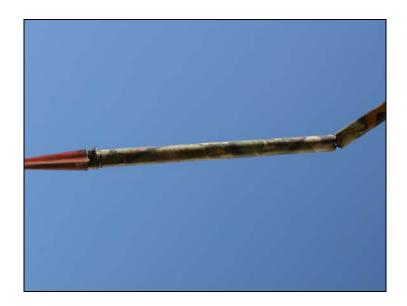
Using a solid reinforcement back of the insert merely shifts the shaft's weak-point further back along the shaft, as shown by this shaft's angular-impact fracture.
