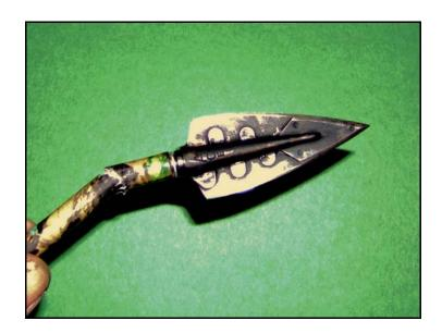
This 1119.5 gr. double-carbon shaft broke behind the aluminum insert, failing to penetrate the entrance rib.
