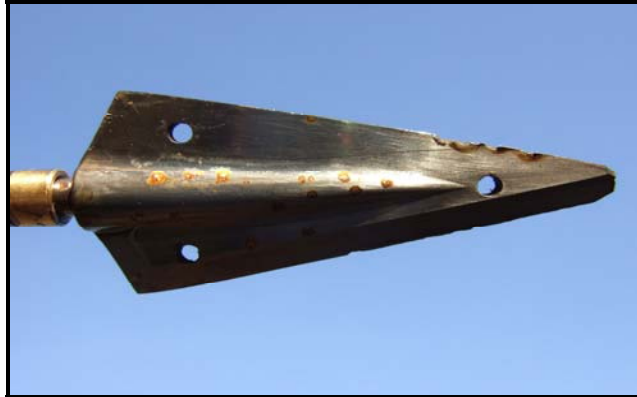
Second set of edge chips on the one, likely over-hardened, prototype Ashby broadhead.
