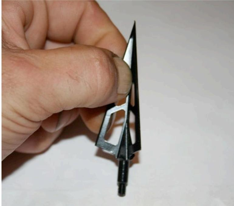
This forward grip also helps in preventing the rear of the blades from flexing as we file or sharpen the broadhead. Now, using **VERY LIGHT PRESSURE**, drag the broadhead backward along the file for 3 or 4 passes on one set of blades. Then have a look at the blades, you'll see that the ink is gone from some areas and still on the blades in other
