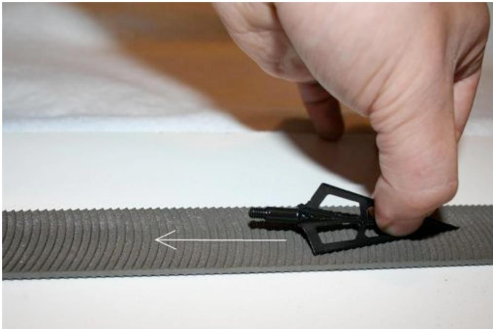
places. It's very likely that you'll have removed more ink/metal from the blade that was below your thumb than from the blade that was below your finger. This is because the knuckle of the thumb is probably locked when sharpening whereas the knuckle of the
